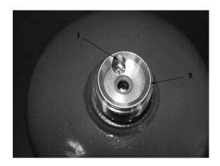
1. Slot for plastic guide & Pressure relief valve
